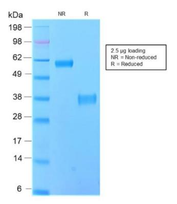
Pr00205 under non-reducing and reducing (DTT) conditions resolved by SDS-PAGE and stained using Coomassie-Blue (representative image).
